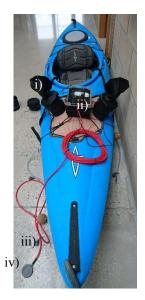
Fig.1: Sonic Kayak system consisting of: i) speakers, ii) box containing electronics, iii) weight and iv) hydrophone
