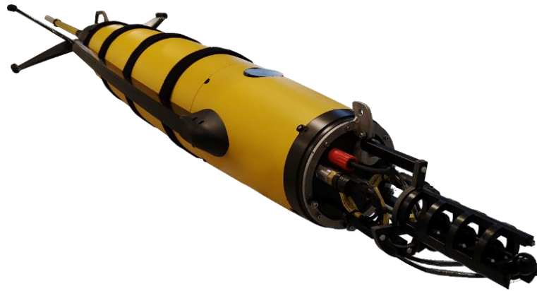
Fig.2: Hydrophones mounted on the glider
