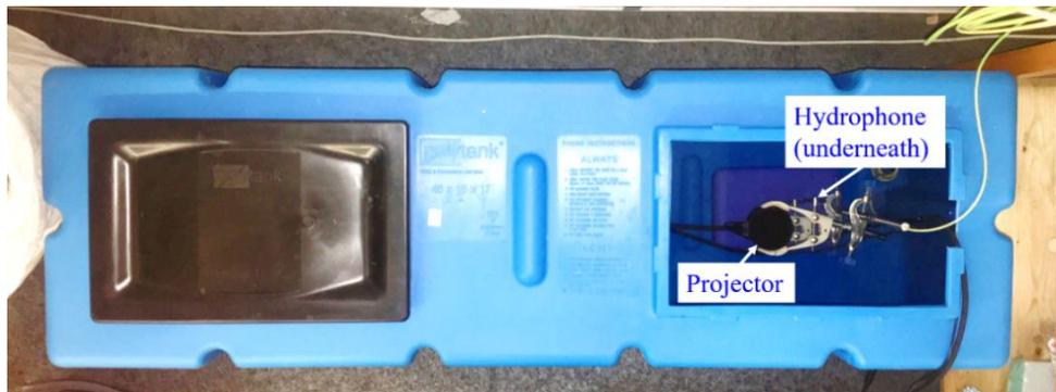
Fig.3: Configuration of the water tank experiments.
