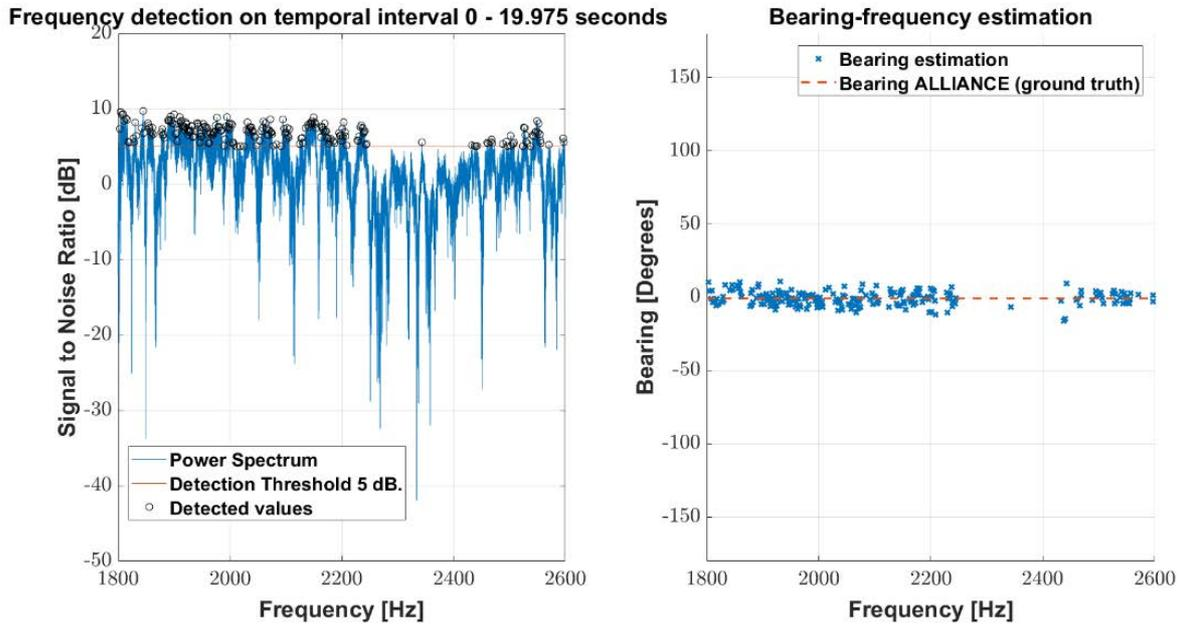
Fig. 2: (Left) Signal to Noise Ratio on the Omni sensor. (Right) Bearing-frequency estimates of a single CAS waveform.
