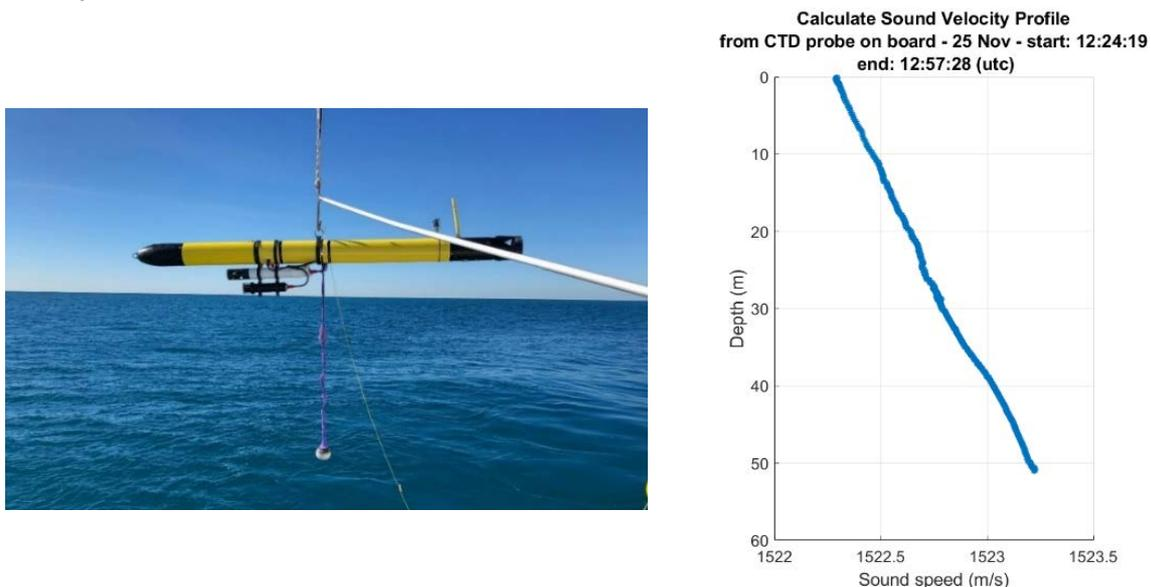
*Fig. 1: (Left) Vehicle deployment. The two payloads: acoustic modem and acoustic vector sensor, are clearly visible. (Right) Sound Speed Profile measured from the CTD probe on board the vehicle.*
