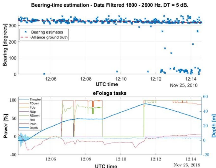
Fig. 5: (Top) Detection contacts and associated bearings. (Bottom) The eFolaga tasks while acquiring data.
