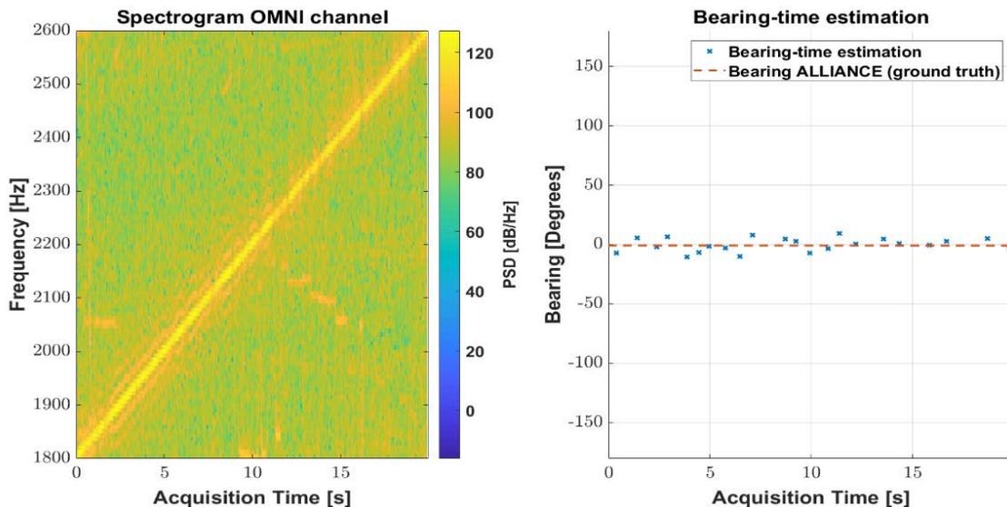
Fig. 3: (Left) Spectrogram of the received signal in which the CAS signal is clearly visible. (Right) Bearing-time estimates of the single CAS.
