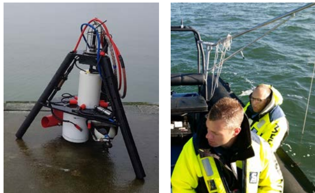
Figure 2: The receiving NILUS bottom node (left) and the onboard crane used for deploying the transmitter (right).
