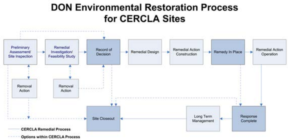
Figure 1 – Generic UXO restoration process covered under the Dept. of Navy (DON) Comprehensive Environmental Response, Compensation, and Liability Act (CERCLA).
