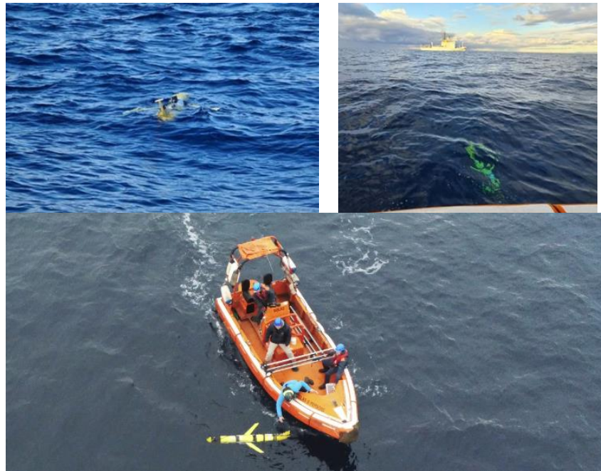
Fig. 2- Buoyancy gliders equipped with AVS.
