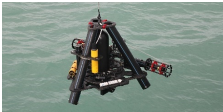
Figure 1: Bottom node equipped with two 3D GeoSpectrum M20-040 AVSs
