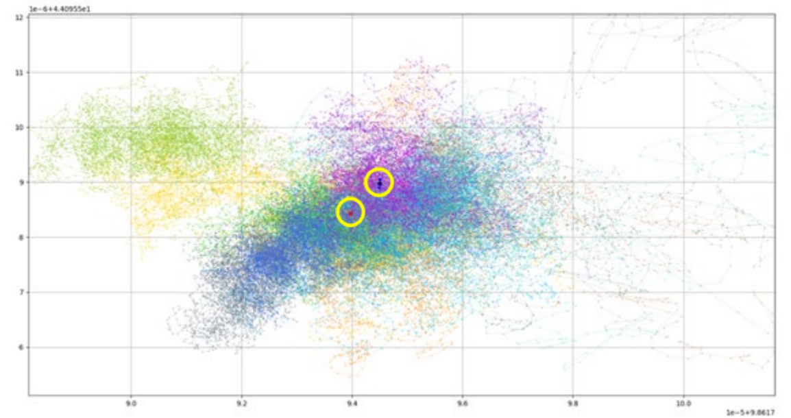
Figure 4 – Positions of the GPS-RTK Float moored atop one of the UXO Targets, sampled at 5Hz over an interval of 3 hours; the data cloud is divided in colour for every 15 minutes; the blue dot is the average position of the GPS-RTK Float; the red dot is the interpolated (“snapshot”) GPS-RTK position recorded at the deployment crane pulley
