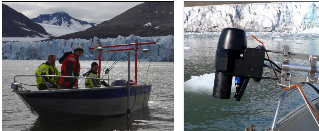
Fig. 2: The survey boat with the T pole mounting of multibeam echosounder (left) and the MBES attached to the pole (right).
