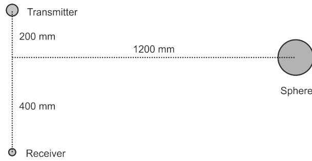
Figure 2: A schematic of the measurement configuration.
