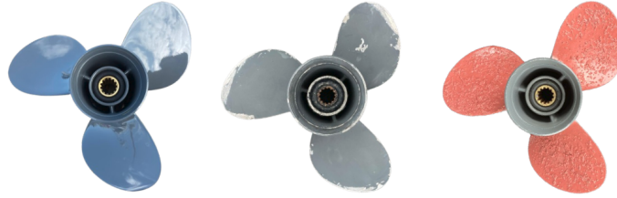
Figure 4: The clean (left), damaged (centre), and artificially roughened (right) propellers.
