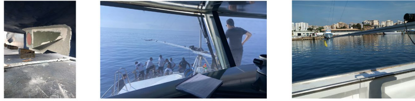
Fig.1: Left: image of echosounder transducer mounted on the starboard side of the boat. Centre: image of rig during sonar calibration. Right: image of rig during echosounder calibration.
