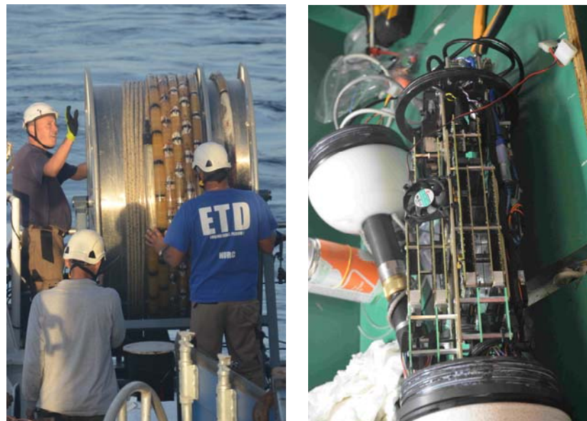
Fig.1: SLICTA ready to be deployed on its storing drum (left) and SLICTA acquisition system and the two lids of the canister (right). Vertically it is possible to see the motherboards which constitute the system and the holding structures.
