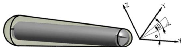
Fig. 3: The BeTTSi model 32, with length 49m, outer shell of 8mm thick steel, small radius 3m, and big radius 5m. The inner body is 46m long with all radii 3m and made of 20mm thick steel. The inner body is air-filled and the volume between the bodies is water-filled.
