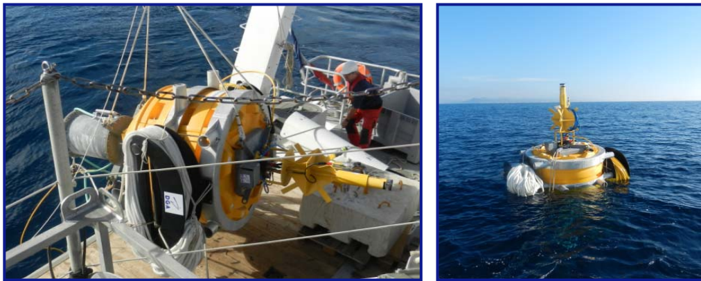
Fig. 2.4: surface buoy for the ALMA passive component: energy and data storage, link to Acoustic Array via electro-optical cable communication link by long range WIFI.
