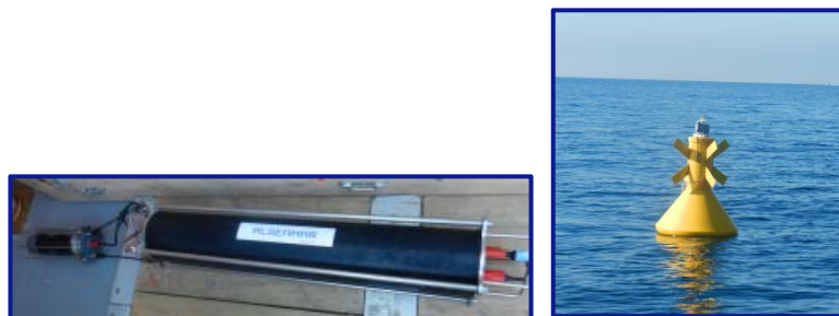
Fig. 2.5: omnidirectional wideband transmitter (realized by ALSEAMAR) and its mooring surface buoy.
