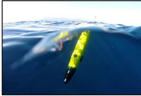
Fig. 3.4: ALSEAMAR “SEA EXPLORER” glider, with CTD payload, deployed on the area during the ALMA 2016 campaign.
