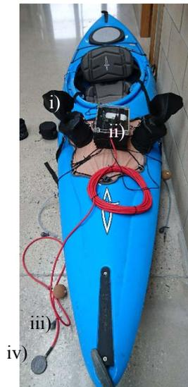
*Fig.1: Sonic Kayak system consisting of: i) speakers, ii) box containing electronics, iii) weight and iv) hydrophone*
