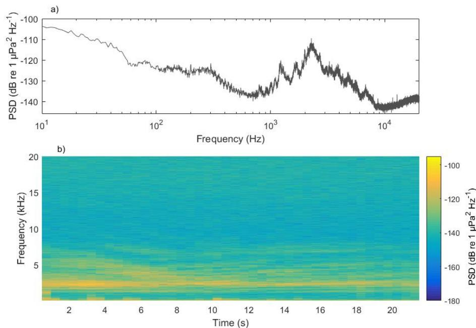
*Fig. 2: a) Mean power spectral density of the vessel noise given in b) giving the average relative sound levels per 1 Hz. b) Spectrogram of vessel noise displaying the sound levels per 1 Hz over time.*
