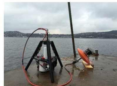
Fig. 1: The NILUS bottom node, with software-defined modem (inside upper Delrin container; wet end in special float shape for stability in currents).
